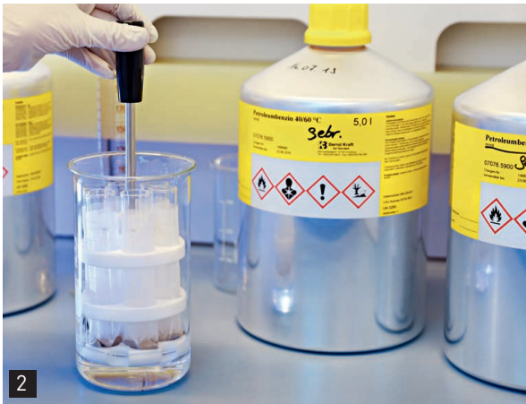
2 Convenient, time-saving degreasing with solvents in the degreasing module. 6 samples can be treated at the same time.
