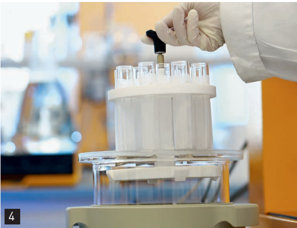
4 The removable handle makes it easier to insert and remove the sample carousel.
