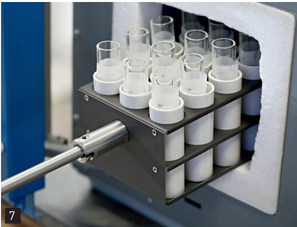
7 The incinerating module with a long handle makes handling of samples easier.
