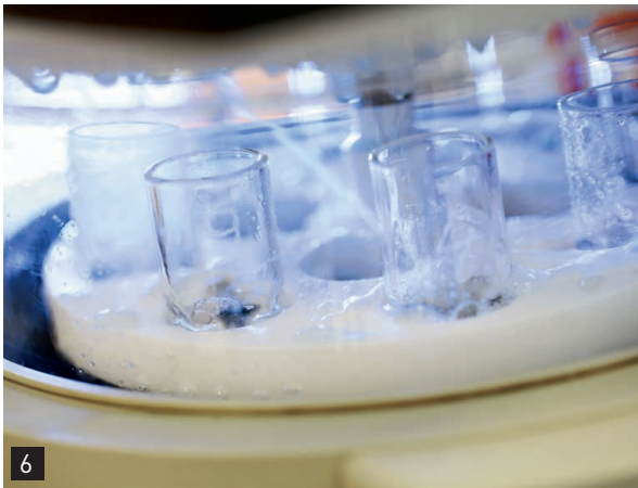
6 The rotating sample carousel ensures optimum bathing of the sample. The rotation is generated by the jet of detergent.
