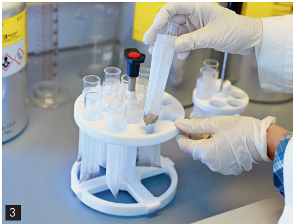
3 When the FibreBags are inserted into the sample carousel, they are automatically clamped firmly in place.
