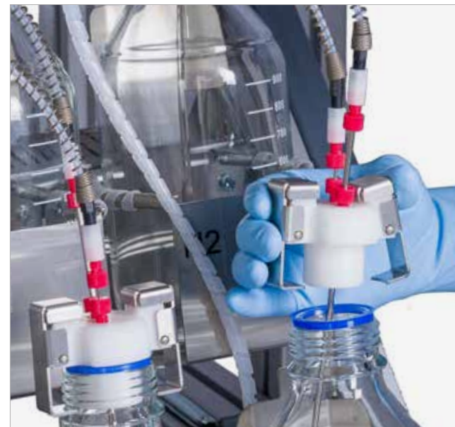
Sample bottle with specially designed closure
